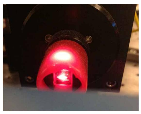
Figure 2: Centering the laser on the input of the isolator
